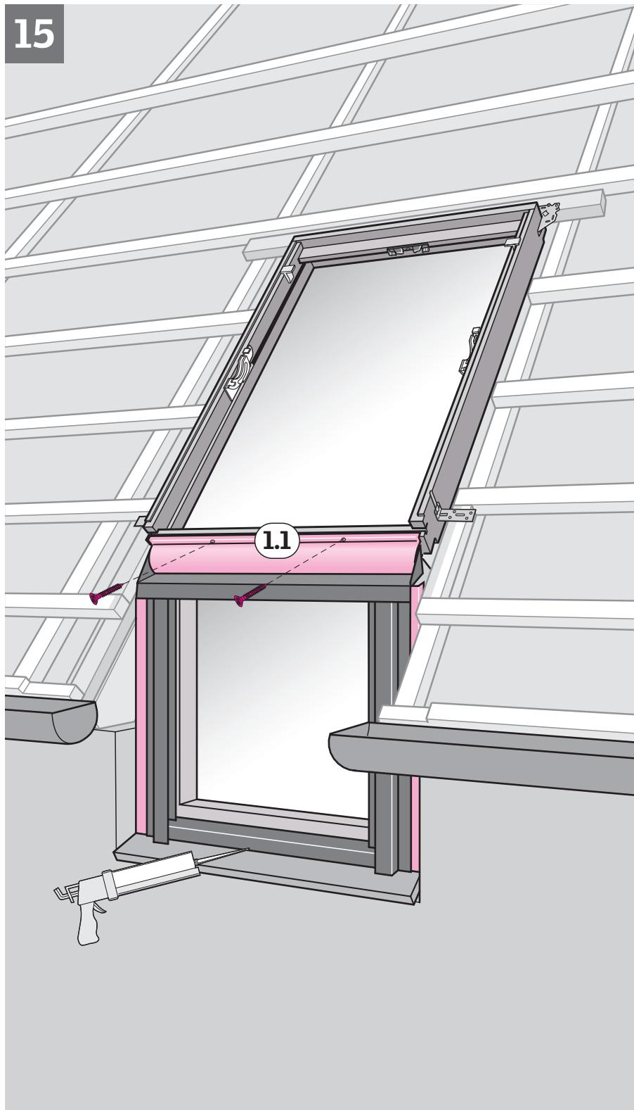
**ENGLISH:** Position cover **1.1** and fix with screws. Pull out side covers against the wall as shown **1**. Connection to underfelt should be carried out as shown in instructions enclosed with upper window. Seal the joint between bottom frame and outer sill with joint sealing **2**.
