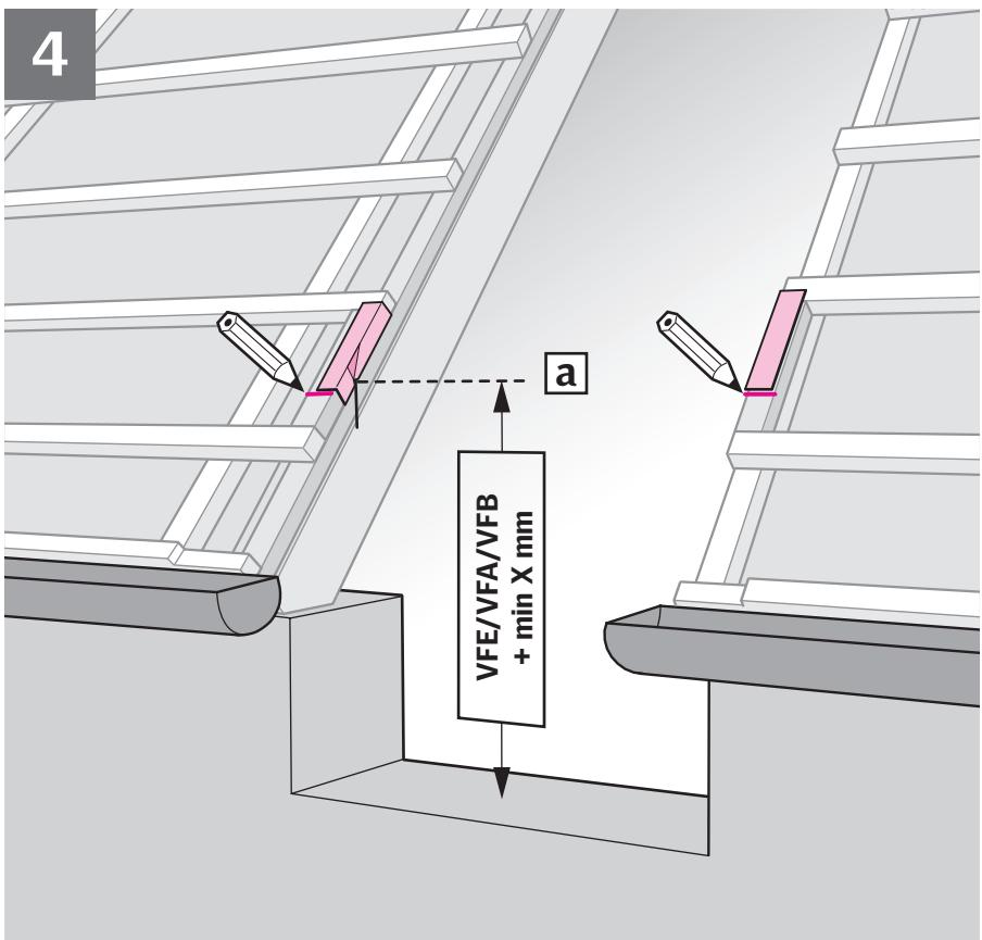
**ENGLISH:** Transfer lines to face of infill battens on both sides using the template. For the position of bottom frame of the roof window see ①. Using the template, check that there is adequate height for the VFE/VFA/VFB **a**.
