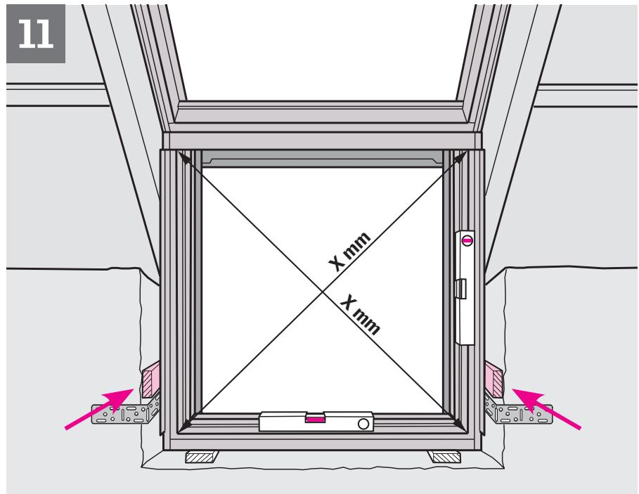
**ENGLISH:** Insert wedges at sides. Ensure that frame is vertical and horizontal. Check diagonal measurements.
