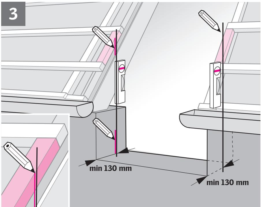
**ENGLISH:** Transfer the distance of min 130 mm from the face of the outer wall to the infill battens on both sides. Mark a vertical line.
