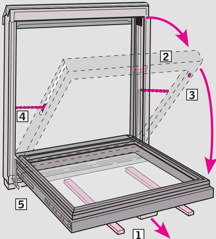
**ENGLISH:** Place packing blocks on a flat surface **1**. Pull handle **2**. If the vertical window element has been fitted with an opening restrictor, turn the button to release mechanism **3**. Press stop and release compound-action arms **4**. Lay sash on packing blocks, then press hinge release and remove sash **5**.
