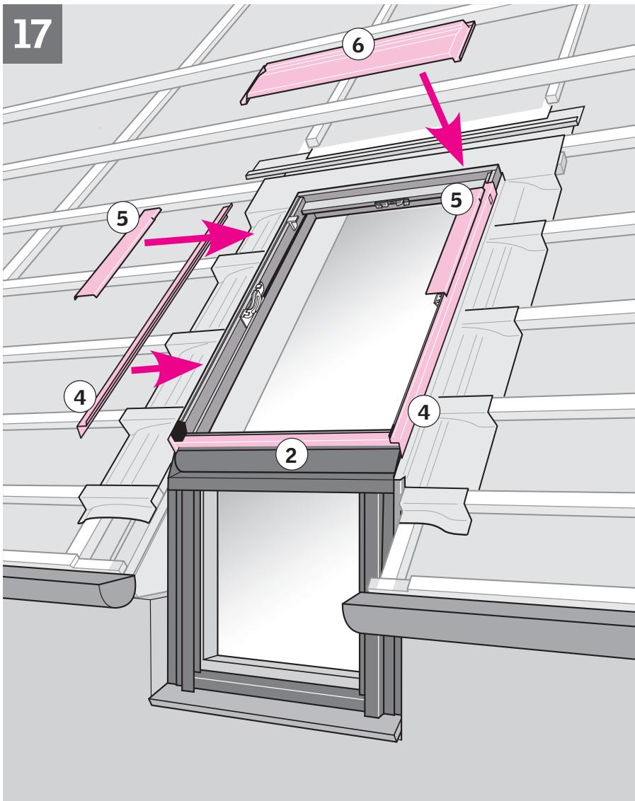
**ENGLISH:** If flashing is not to be installed immediately, fit the covers supplied with the window. Replace sash, if removed earlier, see ill. 18. The push button is automatically released, when the window is closed.
