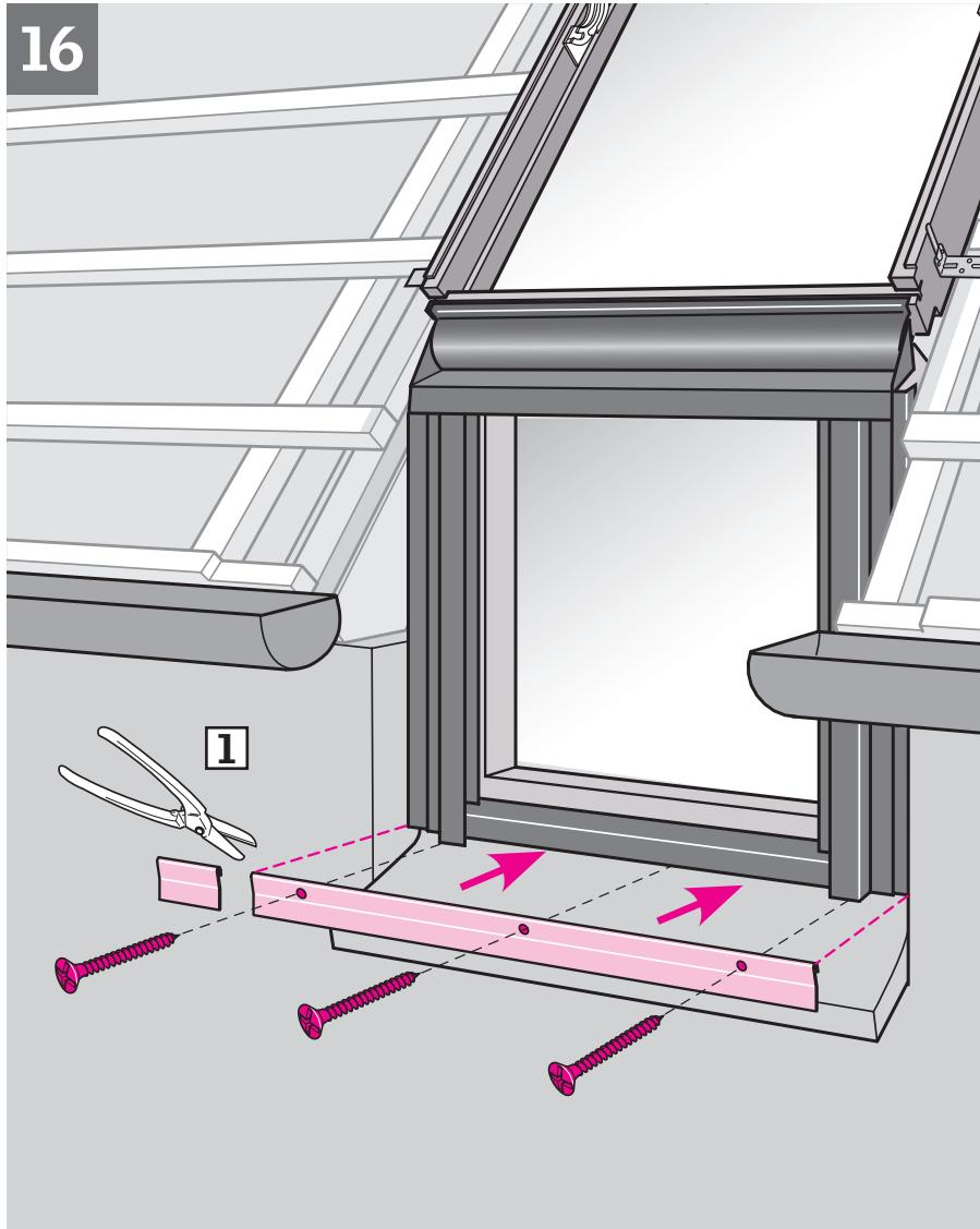
**ENGLISH:** If the vertical window element is supplied with additional bottom frame cover, cut this cover to length **1** and fit it **2**.
