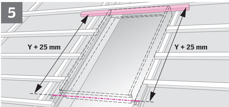
**ENGLISH:** Position and fit installation batten ( $Y + 25 \text{ mm}$ ) from the position for the bottom of the roof window.
