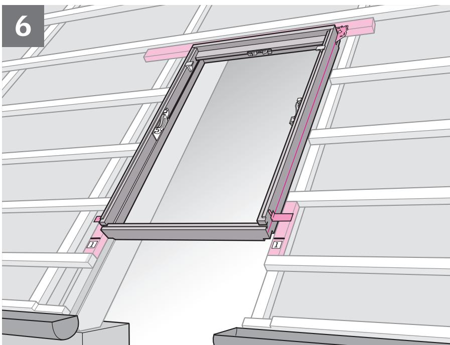
**ENGLISH:** Position roof window. Fix top brackets to installation batten **[a]**. Fix lower brackets to support blocks which must be at the same level as the battens **[b]**. Roof window adjustment: See instructions enclosed with the roof window.
