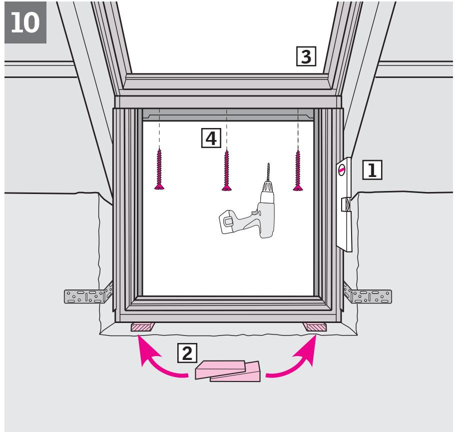
**ENGLISH:** Position frame and check for vertical **1** and support with wedges **2**. Ensure that rebates on both side frames are flush **3**. Drill  $\varnothing$  3 mm hole into roof window and screw frames together **4**. Fit insulating material **5**.
