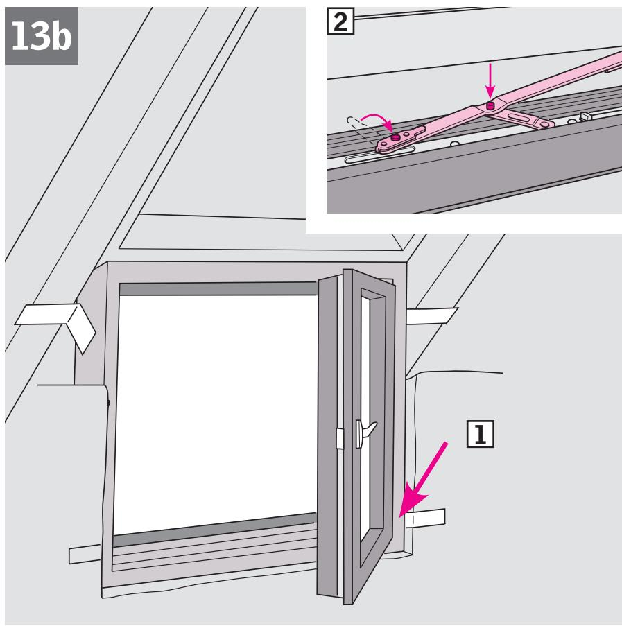
**ENGLISH:** Replace sash: Position sash in frame ensuring that steering pin is positioned in frame fitting **[1]**. Attach and lock fitting arm **[2]**. Close sash **[3]**, **[4]**.
