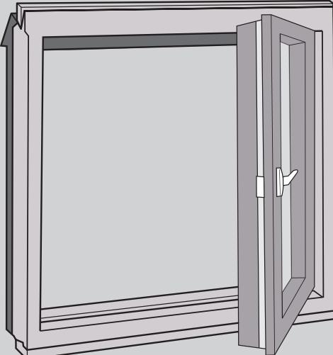
**ENGLISH:** Remove sash: Turn handle and open sash **1**. Turn lock on fitting arm **2**, Release fitting arm and remove the sash **3**, **4**.
