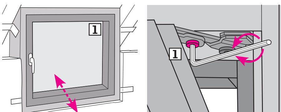
**ENGLISH:** The sash can be adjusted to ensure correct gasket pressure ①, ②.
