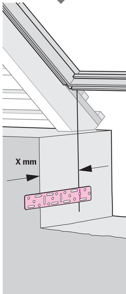
**ENGLISH:** Depending on the distance **X mm**, the fixing brackets are positioned as shown in ill. **8a** or **8b**. Make sure to observe the distance of min 60 mm from the corner to the first screw hole **1**. Transfer the vertical line marked in ill. **3**, to the fixing brackets **2**.
